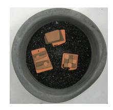
Cover the pieces with more carbon, to the top of the box. Place the box in the kiln, raised on posts.
