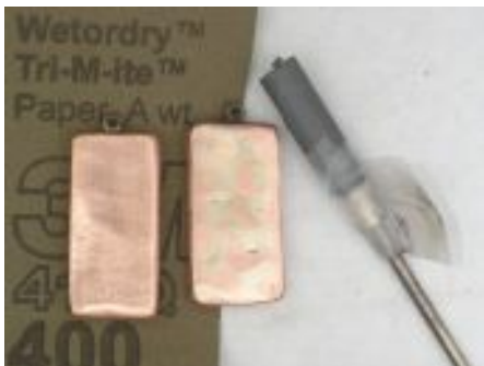
Sanding with 400-grit sandpaper mounted on a straight head slotted mandrel
