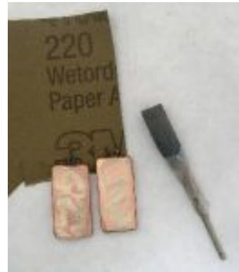
Sanding with 220-grit sandpaper mounted on a straight head slotted mandrel
