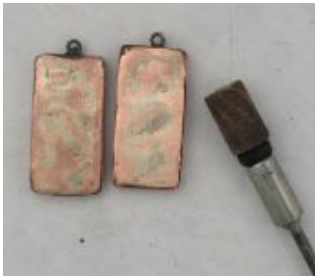
Sanding with a drum mandrel
