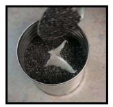
TEST 3D: REPEAT TEST 3C – THIS TIME NO ATMOSPHERE FIRING For this test I am repeating the previous test, only this time I will <u>not</u> do the atmosphere firing first. I want to test my theory that atmosphere firing first is beneficial and helps to prevent the piece from distorting during reduction firing.
